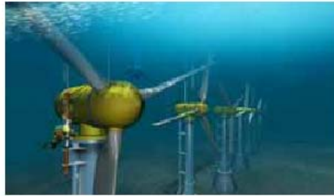
Fig 4 : Graphic depicting Hammerfest Strøm horizontal-axis, ‘water mill’ tidal stream turbine. Turbine propellers consist of 15-16 m blades mounted on towers placed on the sea bed. Tidal currents drive the propellers, with blades automatically adjusting toward the prevailing current. Each propeller is coupled to a subsea generator from which the produced electricity is fed via shore-connecting cables to a transformer and then on into the grid.
