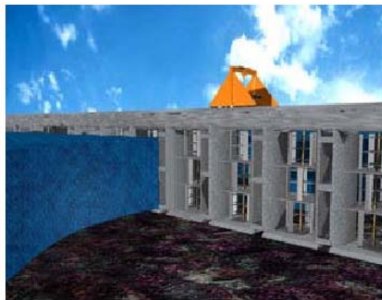
Fig.2 : Cutaway graphic of a ‘mid-range-scale’ (2 x 250 kW) vertical-axis tidal turbine.
