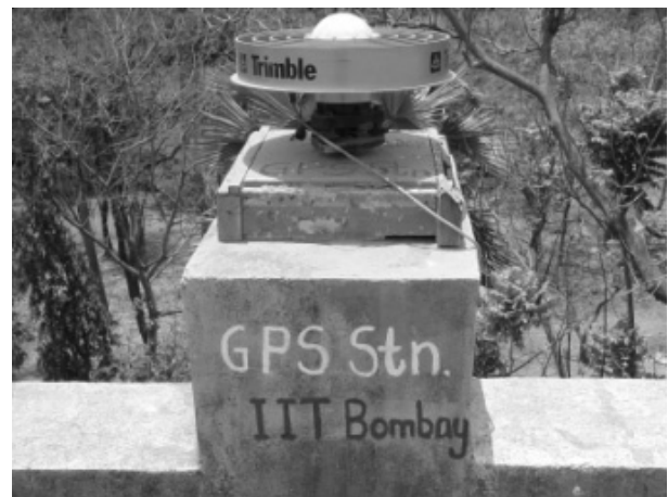
Fig. 3. IITB Permanent GPS Station
