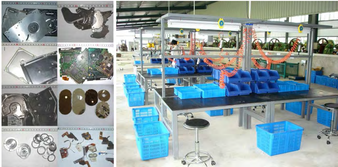
Figure 6: Deep-level manual dismantling of hard disks (left) and dismantling table with pneumatic tools (right)
