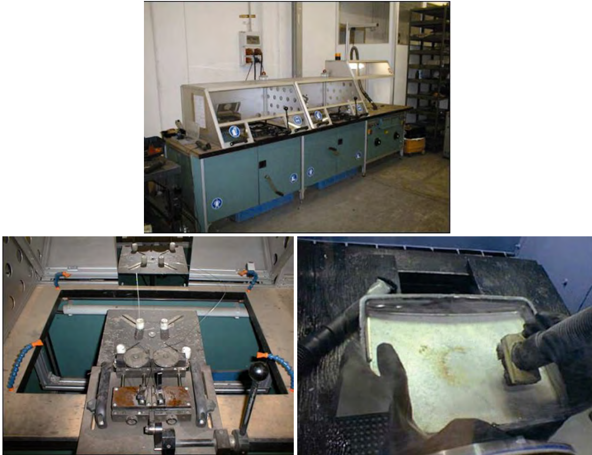
Figure 7: Semi-automatic line for cutting (hot wire) of CRT and removal of coatings
